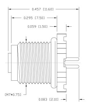
NOTE: MATERIAL HOUSING: PBT UL94V-0, BLACK CONTACT: BRASS NUT: BRASS BRASS SHELL: □-RING: NBR, BLACK FINISH CONTACT: GOLD PLATED OVER 504" NICKEL NUT: NICKEL PLATED NICKEL PLATED SHELL: ELECTRICAL RATED CURRENT: 1A 60V RATED VOLTAGE: INSULATION RESISTANCE: 100 MOhms MIN. CONTACT RESISTANCE: 10 mOhms MAX.. WATER PROOF: IP67 ENVIRONMENT OPERATION TEMPERATURE: -40°C TD +85°C
