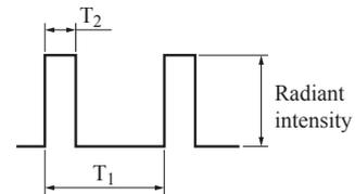
**Fig.4 Output Waveform Specification(Transmitter side)**
