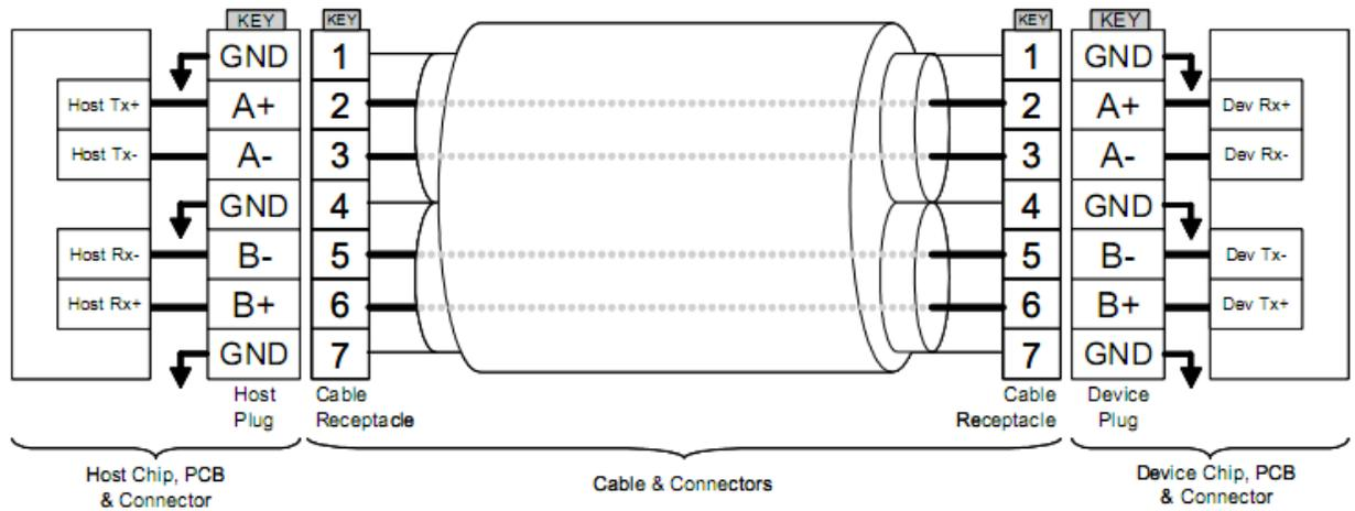
**Figure 3-2** SATA Cable / Connector Connection Diagram
