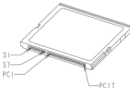
**Figure 3-1** Pin Assignment
