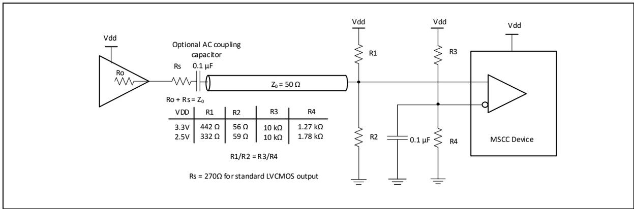
**Figure 7. Input driven by a single ended output**
