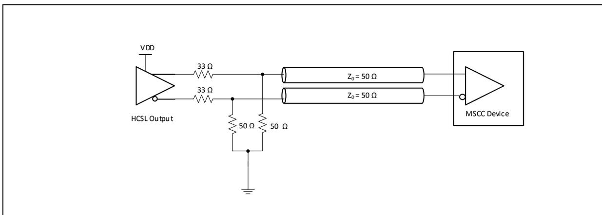
**Figure 3. Input driven by source terminated HCSL**
