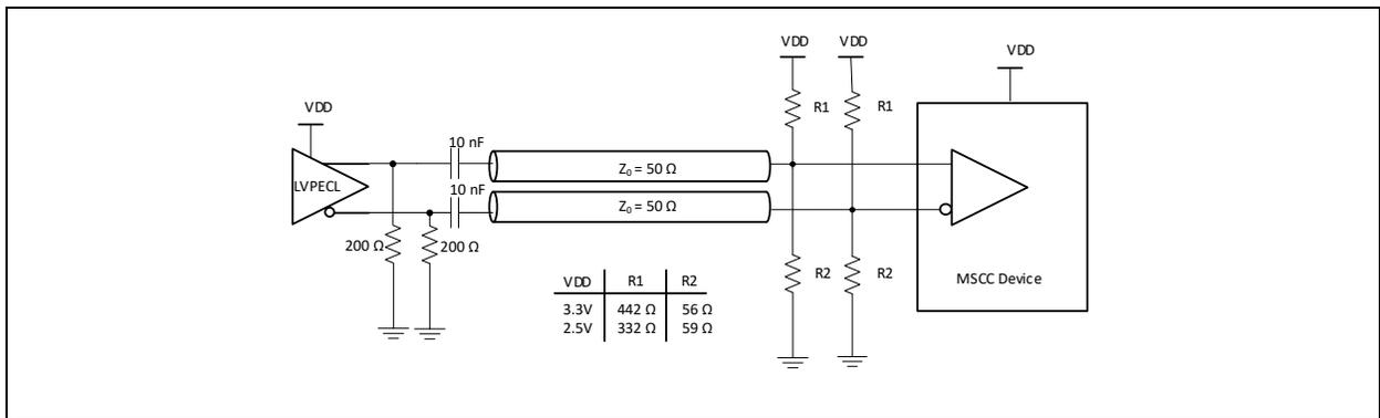
**Figure 5. Input driven by AC coupled LVPECL output**
