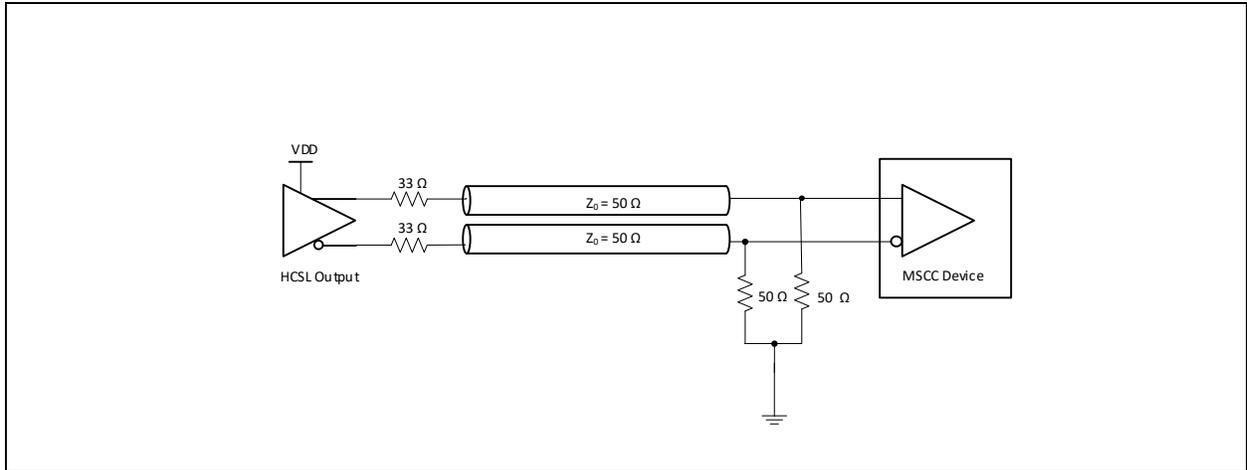
**Figure 4. Input driven by receiver terminated HCSL**
