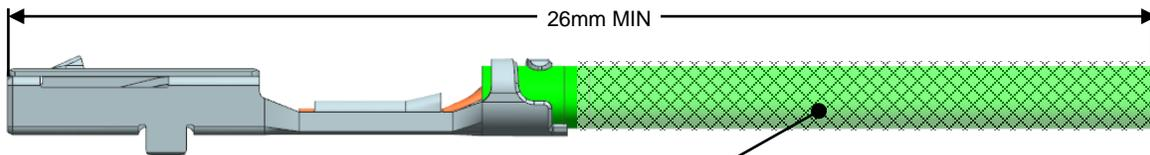
No scratches, grooves or dents permitted on this region of the wire after crimping
