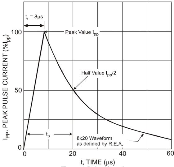
Figure 3 Pulse Waveform
