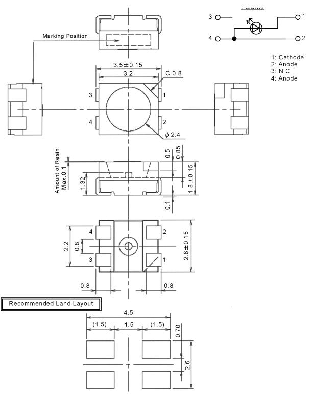
(Note1) Tolerance unless specified: ±0.1 mm.
