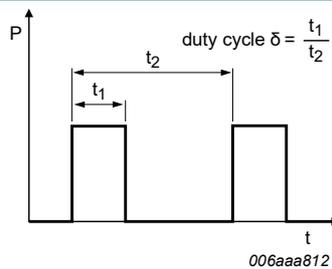
Fig. 14. Duty cycle definition
