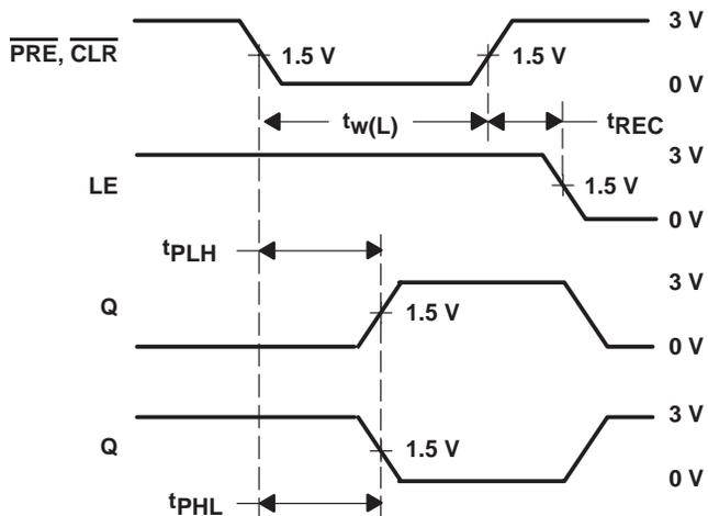
Figure 1.  $\overline{\text{CLR}}$  and  $\overline{\text{PRE}}$  Pulse Duration,  $\overline{\text{CLR}}$  and  $\overline{\text{PRE}}$  to Output Delay, and  $\overline{\text{CLR}}$  and  $\overline{\text{PRE}}$  to Latch-Enable Recovery Time
