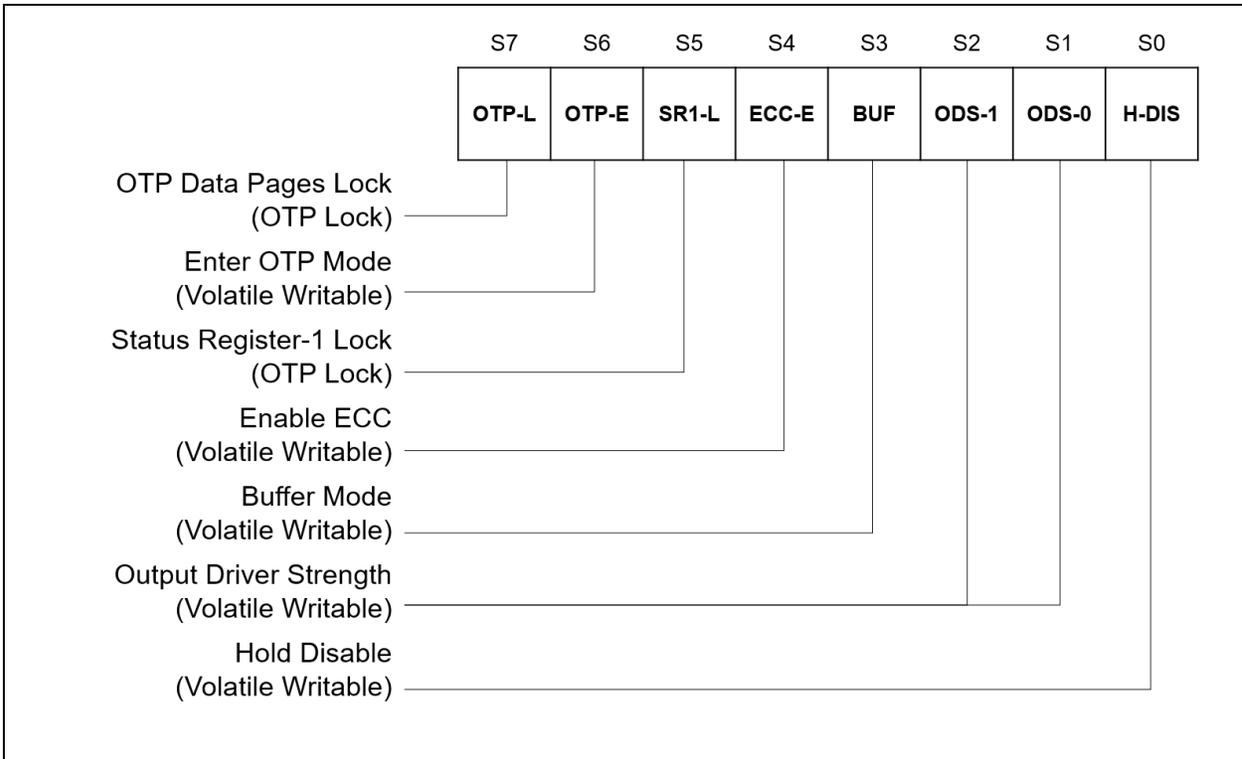
Figure 4b. Configuration Register / Status Register-2 (Address Bxh)
