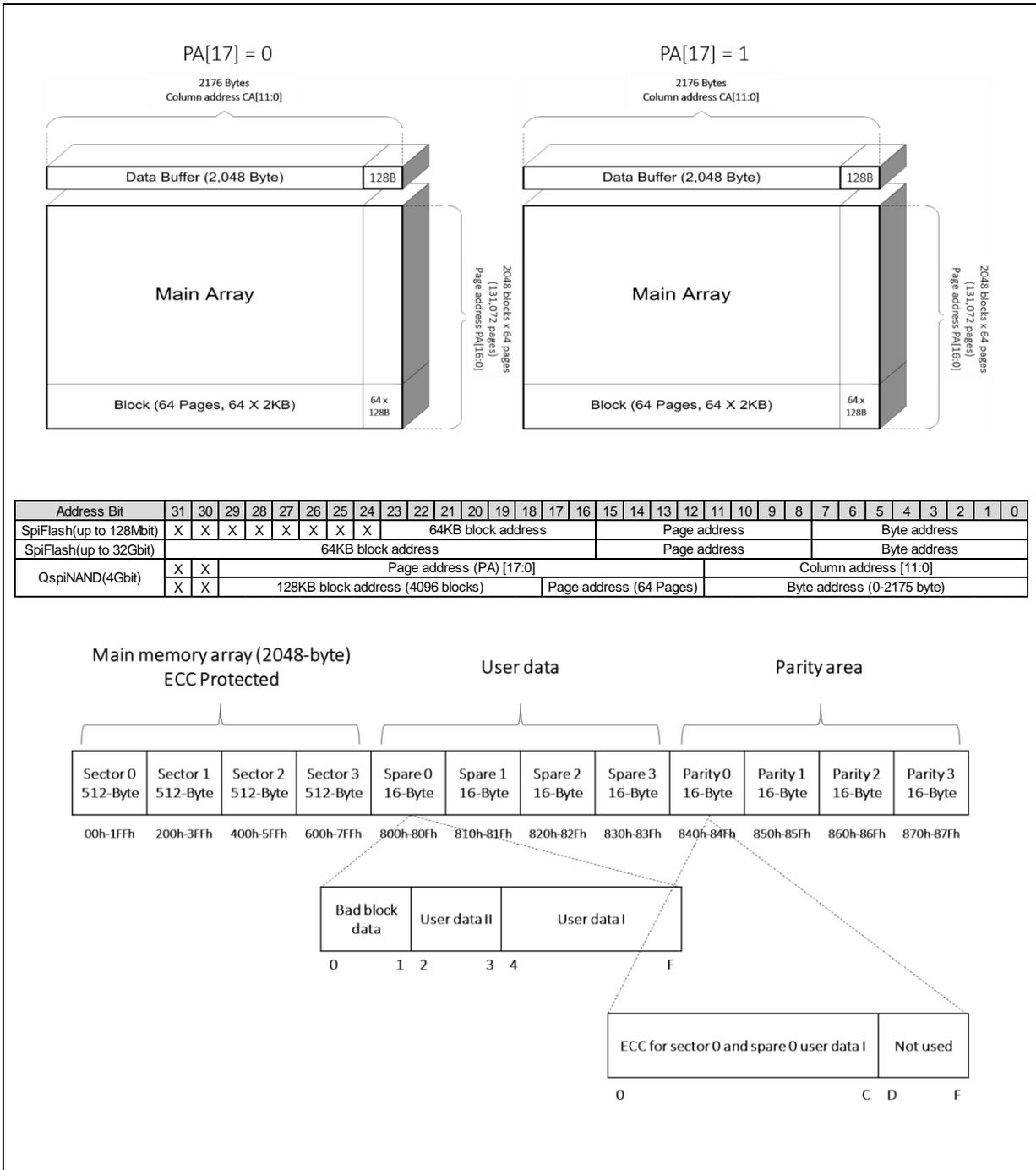
Figure 2. W25N04KV Flash Memory Architecture and Addressing
