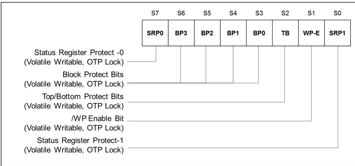
Figure 4a. Protection Register / Status Register-1 (Address Axh)
