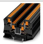
Feed-through terminal block, nom. voltage: 1000 V, nominal current: 41 A, connection method: Push-in connection, Rated cross section: 6 mm², cross section: 0.5 mm² - 10 mm², mounting type: NS 35/7,5, NS 35/15, color: black
