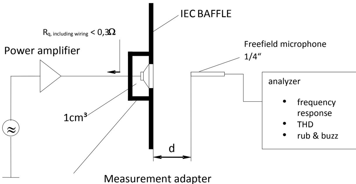
Measurement signal: Logarithmic sine sweep, 1.5s, 22kHz-180Hz
