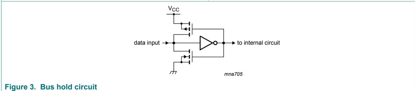
Figure 3. Bus hold circuit
