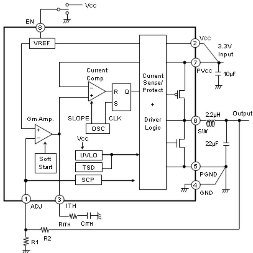
Fig.3 Block diagram
