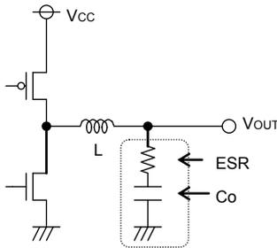
Fig.29 Output capacitor
