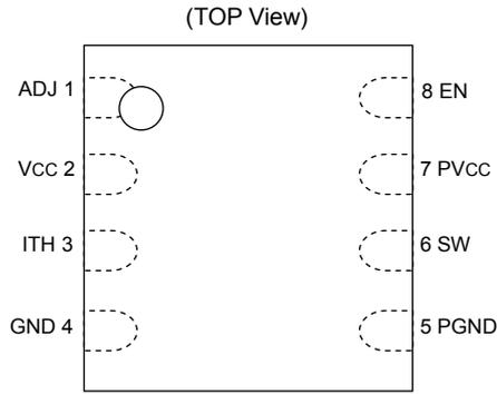
Fig.2 Pin Configuration
