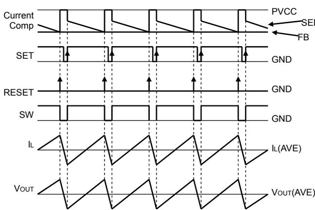
Fig.20 PWM switching timing chart
