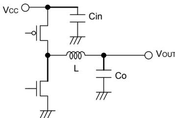
Fig.30 Input capacitor
