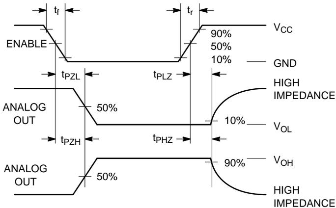
Figure 15. Propagation Delays, Enable to Analog Out
