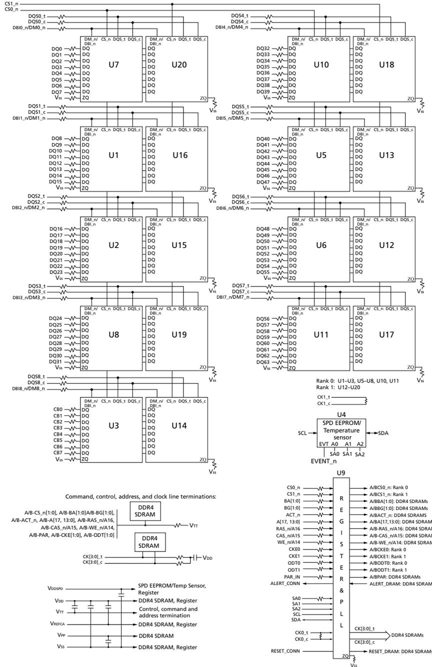
Note: 1. The ZQ ball on each DDR4 component is connected to an external 240Ω ±1% resistor that is tied to ground. It is used for the calibration of the component's ODT and output driver.
