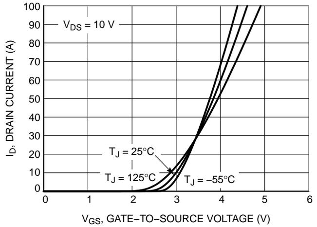
Figure 2. Transfer Characteristics
