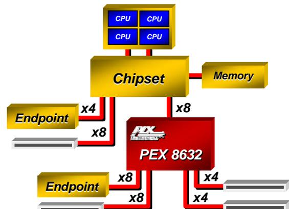
**Figure 3. Fan-in/out Usage**
