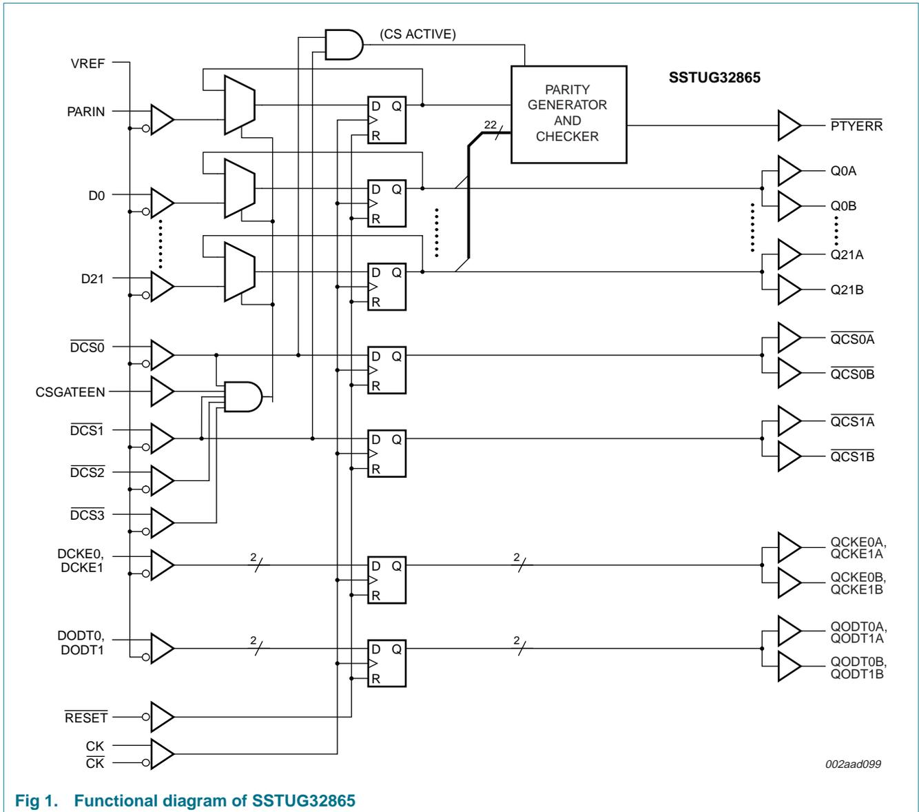
**Fig 1. Functional diagram of SSTUG32865**
