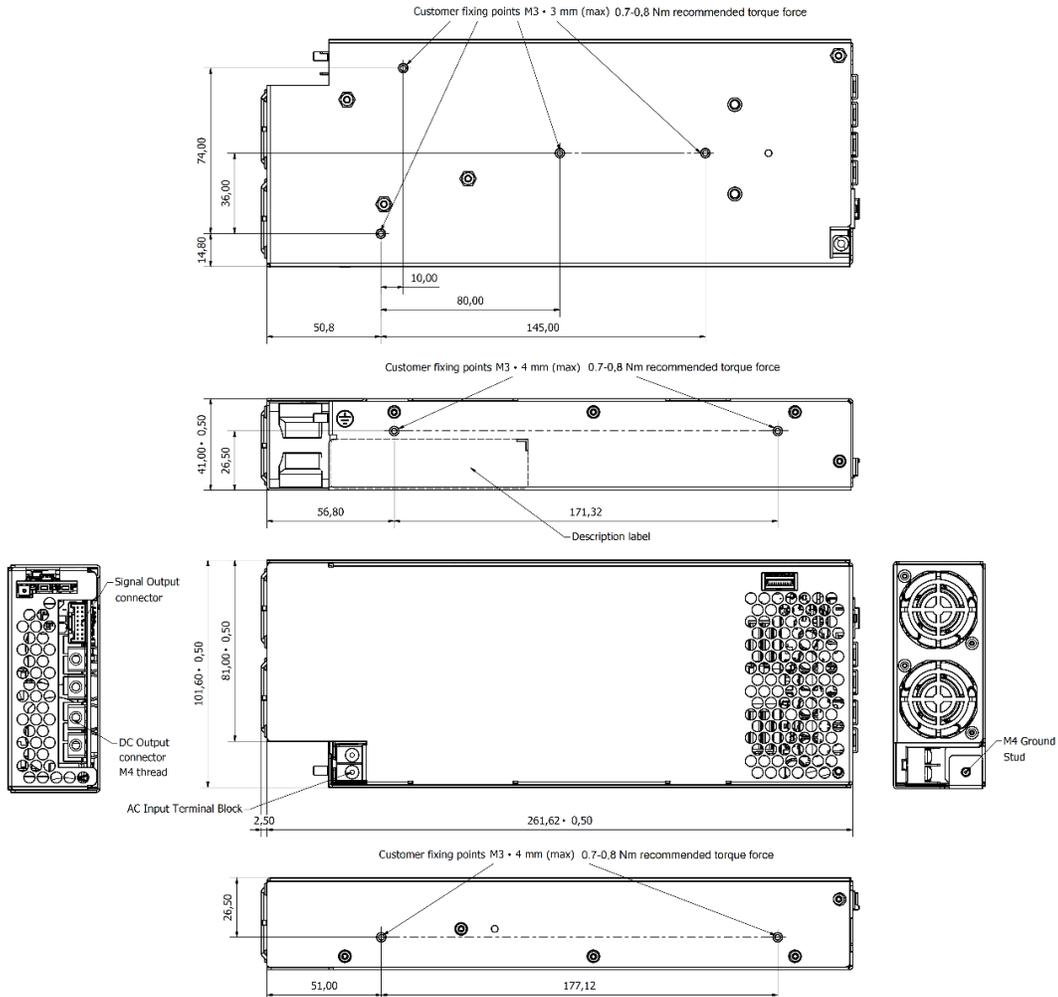
Figure 7. Mechanical Drawing - ABE1200-1T24 / ABE1200-1T48 Models
