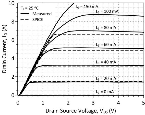
**Figure 1: Typical Output Characteristics at 25 °C**
