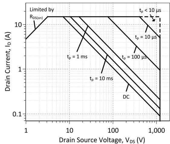
**Figure 18: Forward Bias Safe Operating Area at T<sub>C</sub> = 25 °C**
