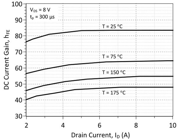
**Figure 4: DC Current Gain vs. Drain Current**
