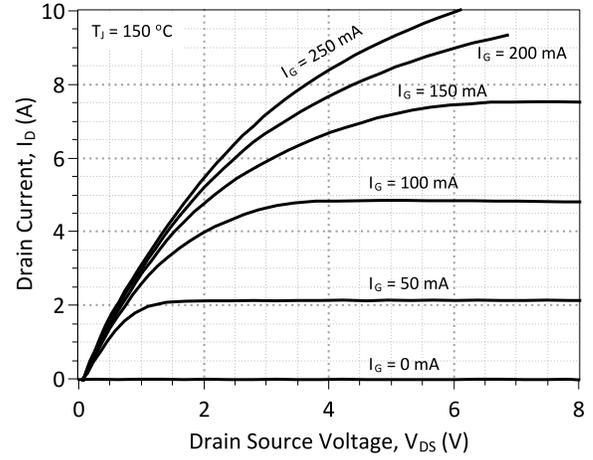
**Figure 2: Typical Output Characteristics at 150 °C**
