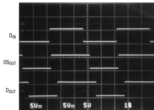
OS<sub>OUT</sub> AND D<sub>OUT</sub> LOADED WITH 15pF SCOPE PROBE
