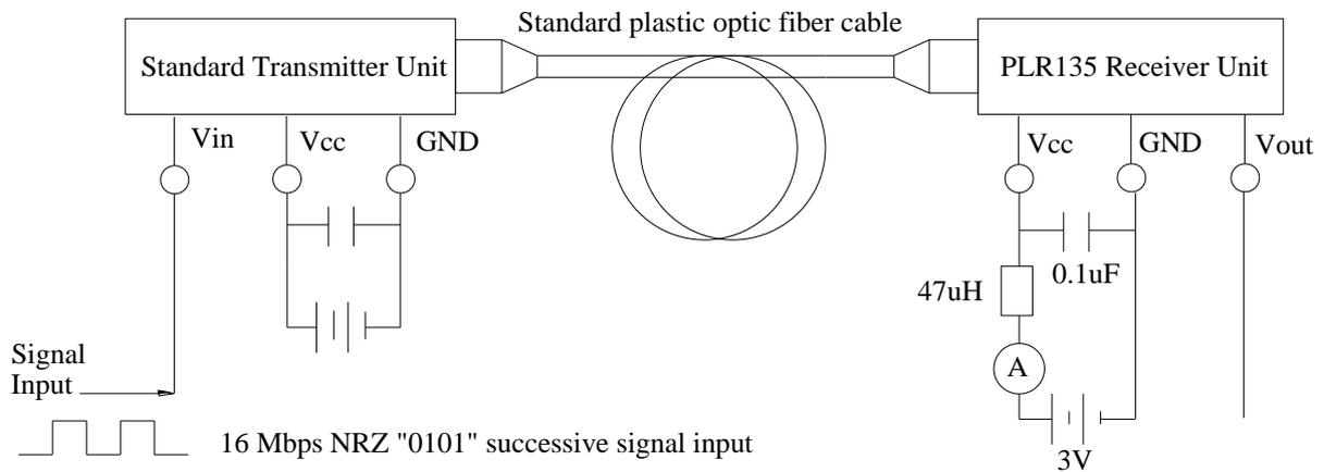
\*Fig.3 Measuring Method of Output Voltage, Pulse and Jitter
