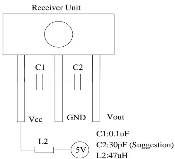
Note: For having good coupling, the C1,C2 capacitor must be placed within 7mm
