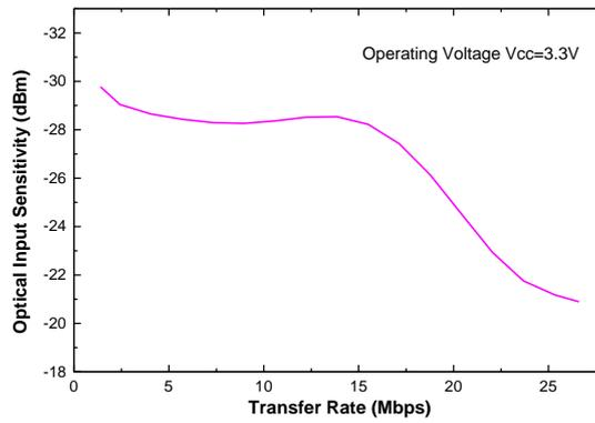
**Note:** Before using the PLR135 device, please confirm the minimum sensitivity at different operating voltage and transmission rate.
