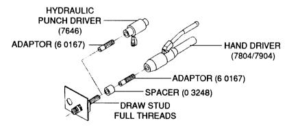
**NOTE:** Seat Adaptor fully into Hydraulic Driver. Seat Draw Stud fully into Adaptor.
