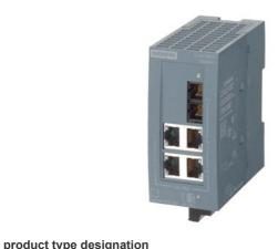
SCALANCE XB004-1LD unmanaged Industrial Ethernet Switch for 10/100 Mbit/s; for setting up small star and line topologies; LED diagnostics, IP20, 24 V AC/DC power supply, with 4x 10/100 Mbit/s twisted pair ports with RJ45 sockets; 1 x 100 Mbit/s single-mode glass fiber-optic cable port with SC socket; manual available as a download .
