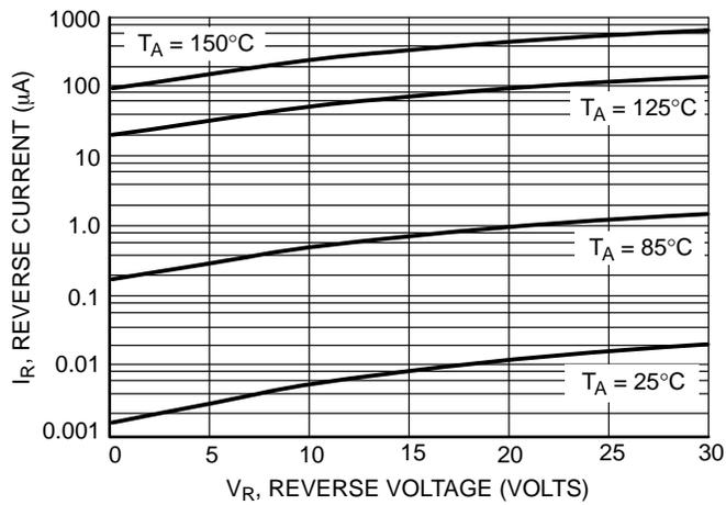
**Figure 3. Leakage Current**
