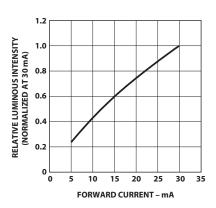
Figure 4. Relative intensity vs. forward current (InGaN)
