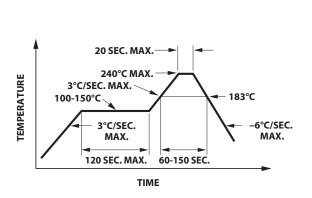
Figure 9a. Recommended SnPb reflow soldering profile
