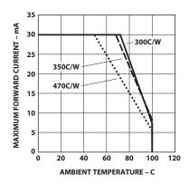
Figure 5b. Maximum forward current vs. ambient temperature, derated based on  $T_J$ max =  $110^{\circ}$ C (InGaN)
