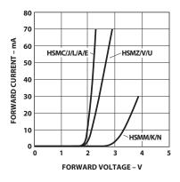
Figure 2. Forward current vs. forward voltage
