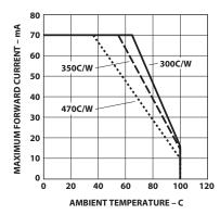
Figure 5a. Maximum forward current vs. ambient temperature, derated based on T<sub>J</sub>max = 110°C (AlInGaP)
