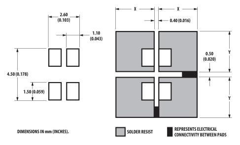
Figure 8a. Recommended soldering pad pattern
