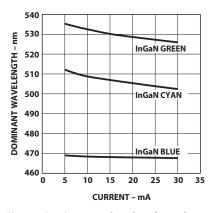
Figure 6. Dominant wavelength vs. forward current – InGaN devices
