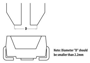
Figure 11. Recommended Pick and Place Nozzle Size for InGaN Family
