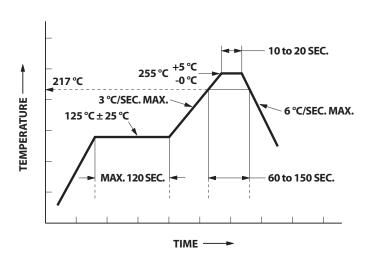
Figure 9b. Recommended Pb-free reflow soldering profile.
