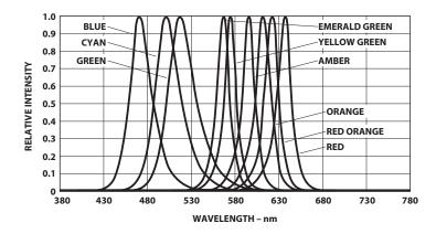
Figure 1. Relative intensity vs. wavelength
