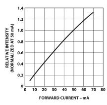
Figure 3. Relative intensity vs. forward current (AlInGaP)
