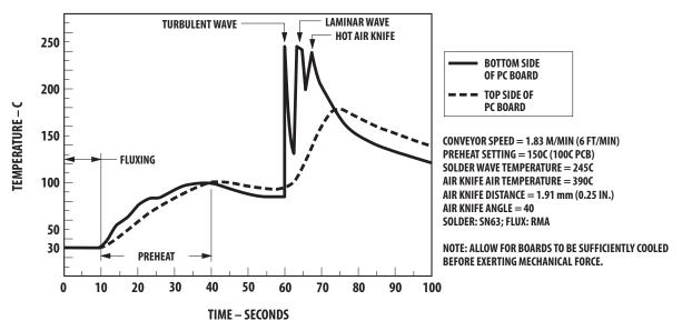
Figure 10. Recommended wave soldering profile
