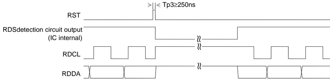
Note: RDCL and RDDA outputs keep high level after input of RST until RDS detection circuit output is detected.
