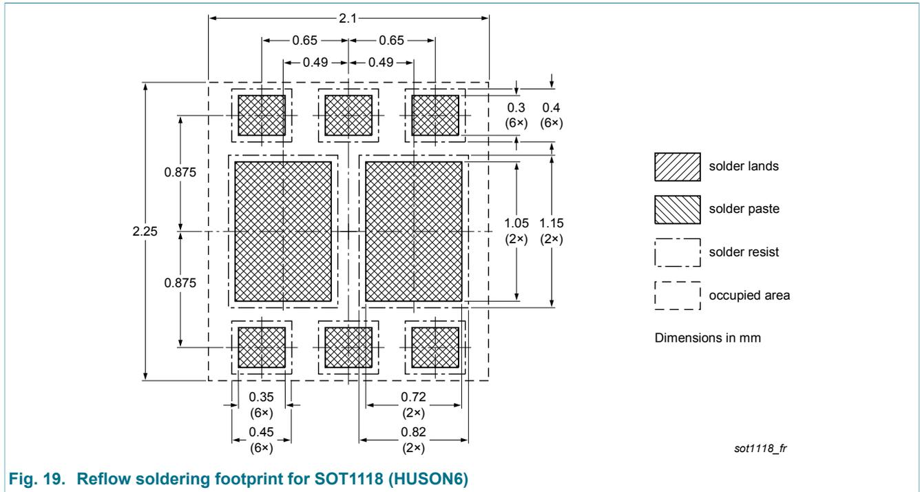
Fig. 19. Reflow soldering footprint for SOT1118 (HUSON6)
