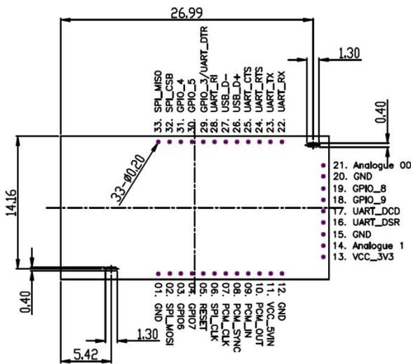
Figure 6-3: BT7xx Mechanical Drawing
