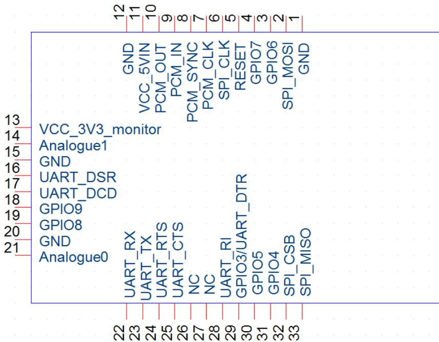
Figure 2-2: BT740-Sx module pin-out (Top View)
