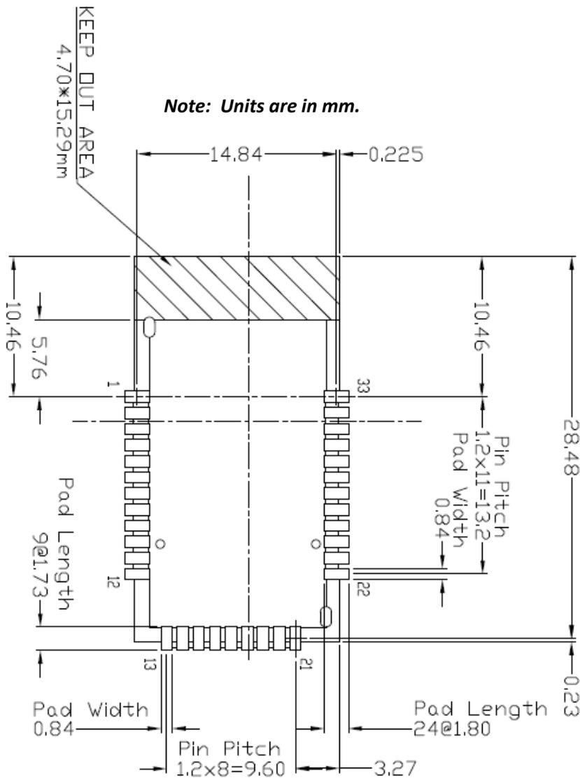
Figure 6-4: PCB Land Pattern and Antenna Keep-out for BT740-SA
