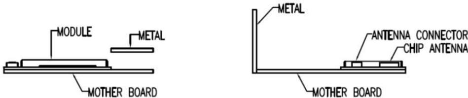
Figure 5-3: Recommended BT740-SA placement on host PCB and proximity to metal cover
