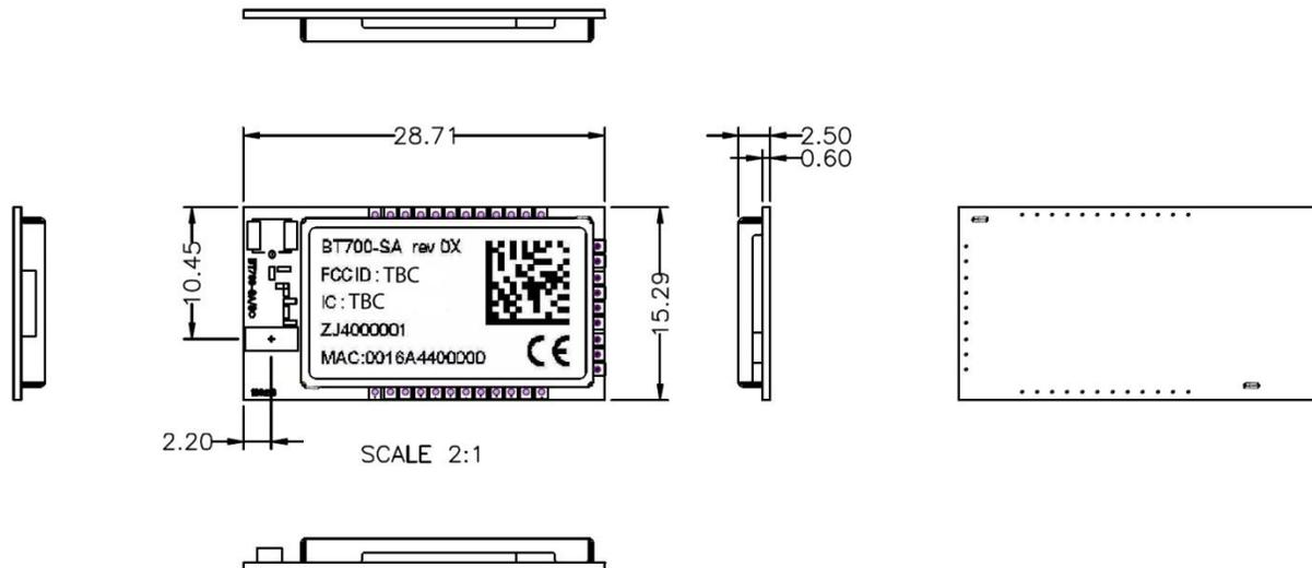
Figure 6-2: BT740-SA mechanical details
