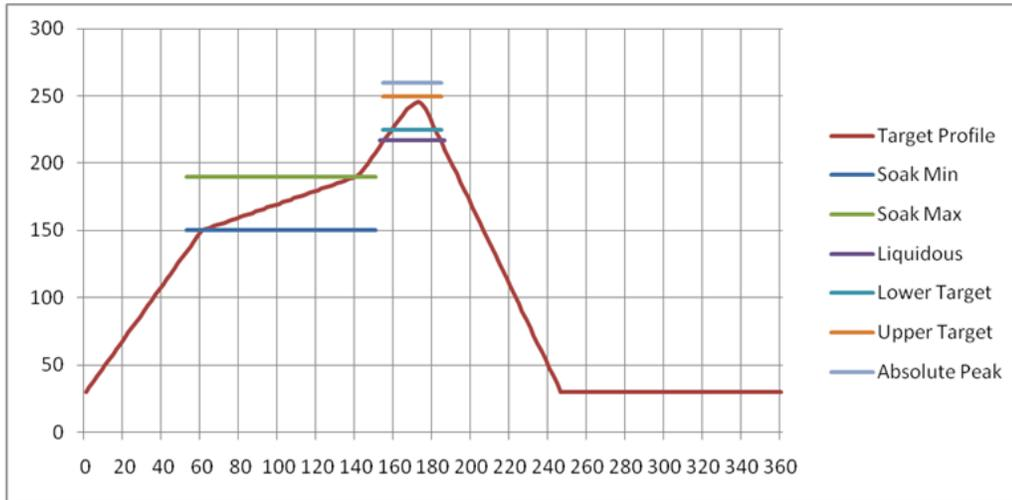
**Figure 7-2: Recommended Reflow Temperature**
