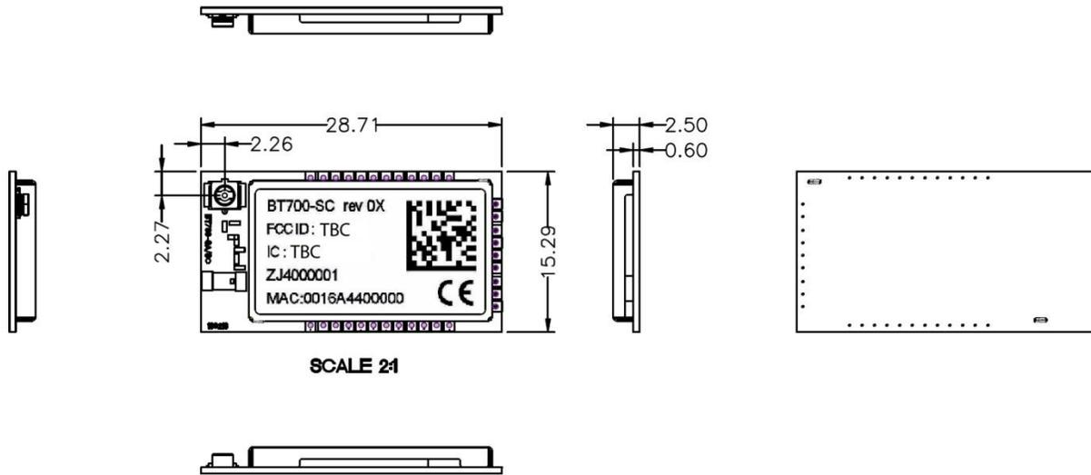
Figure 6-1: BT740-SC mechanical details
