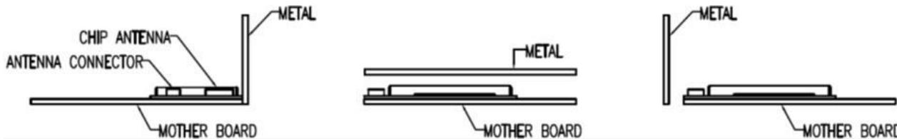
Figure 5-4: Not recommended BT740-SA placement on host PCB and proximity to metal cover
