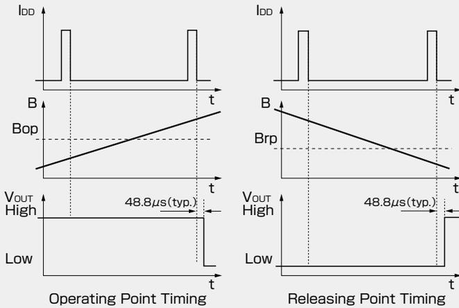
This Hall effect IC's output is held as internal data just before the internal circuit turns OFF ( $I_{DD}$  OFF). And after 48.8  $\mu$ s, the output changes.
