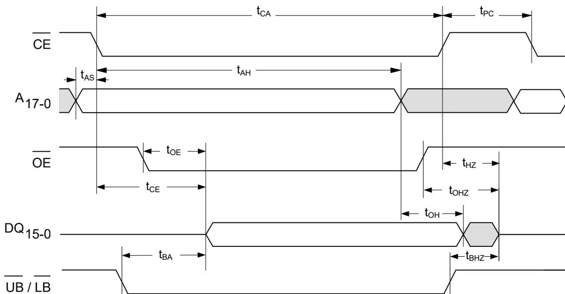
Figure 10. Page Mode Read Cycle Timing <sup>[9]</sup>
