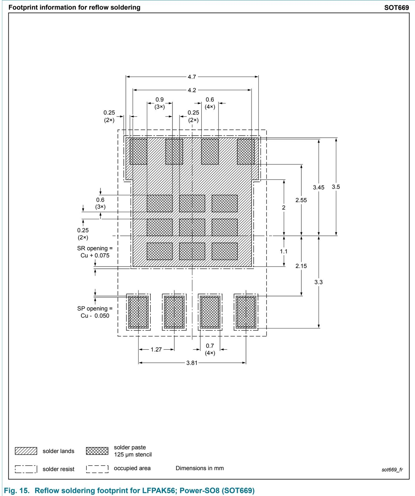
Fig. 15. Reflow soldering footprint for LFPAK56; Power-SO8 (SOT669)
