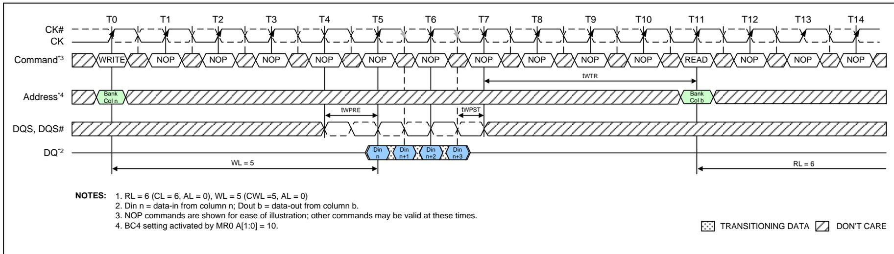
Figure 52 – WRITE (BC4) to READ (BC4)
