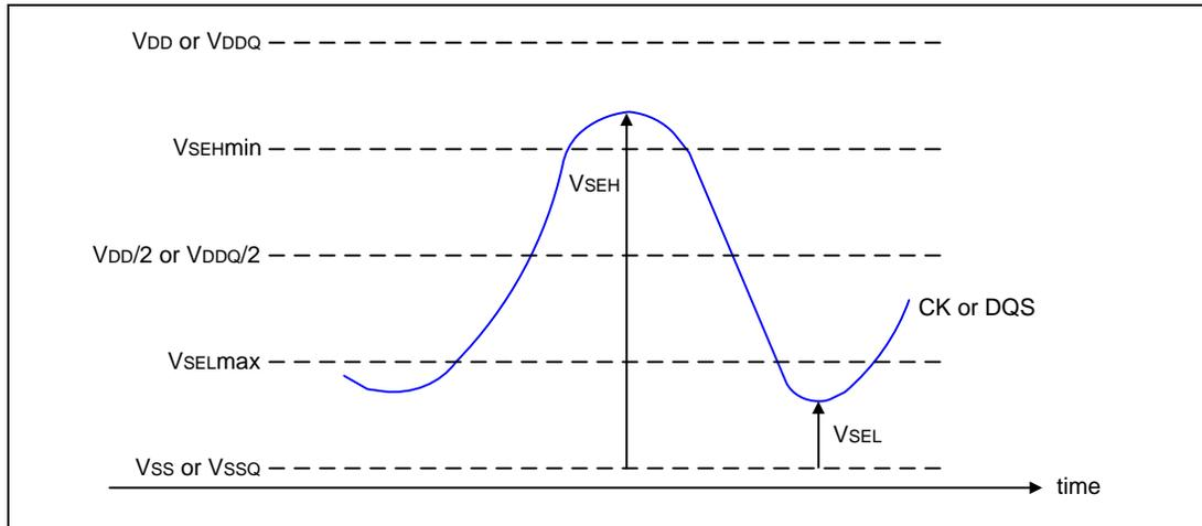
**Figure 91 – Single-ended requirement for differential signals**
