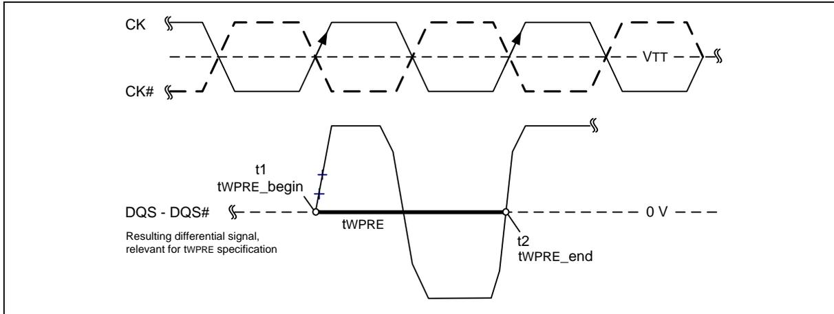
**Figure 41 – Method for calculating tWPRE transitions and endpoints**
