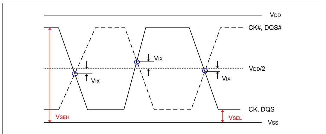
**Figure 92 –  $V_{ix}$  Definition**
