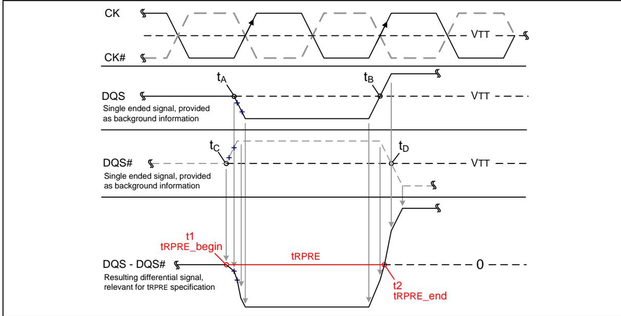
Figure 27 – Method for calculating tRPRE transitions and endpoints
