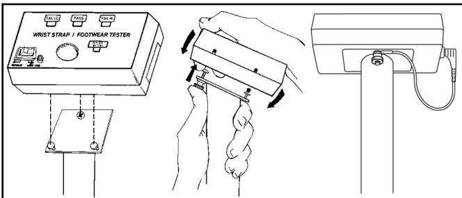
Figure 8. Installing the Combo Tester to the pedestal
