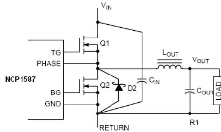
**Figure 12. Components to be Considered for Layout Specifications**
