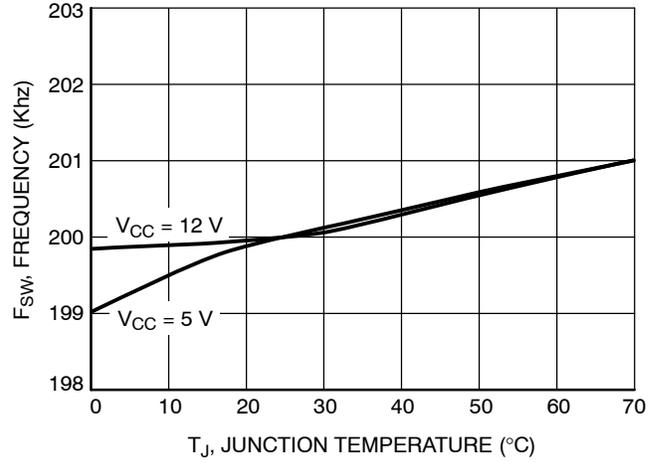
Figure 4. Oscillator Frequency ( $F_{SW}$ ) vs. Temperature
