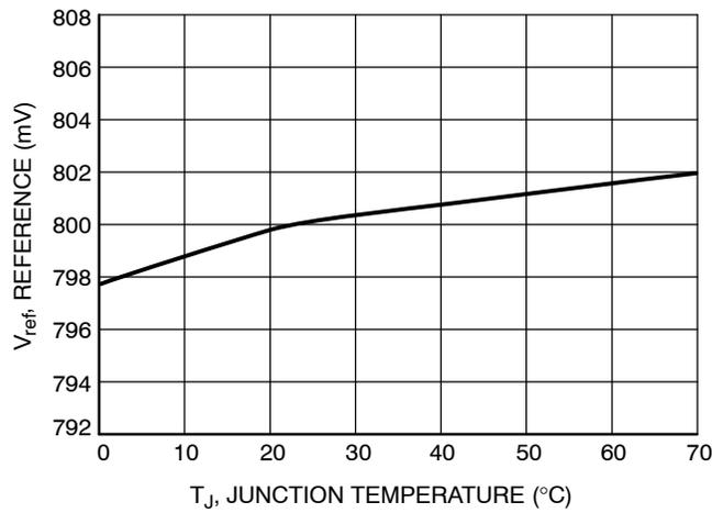
Figure 7. Reference Voltage ( $V_{ref}$ ) vs. Temperature
