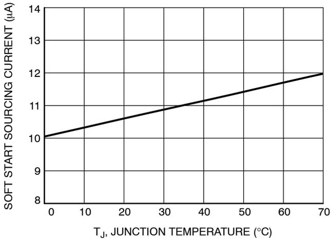
Figure 5. Soft Start Sourcing Current vs. Temperature
