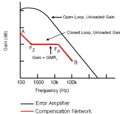
**Figure 11. Gain Plot of the Error Amplifier**
