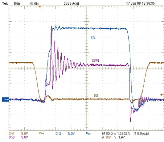
Figure 16. Gate Waveforms 20 A Load Sustaining
