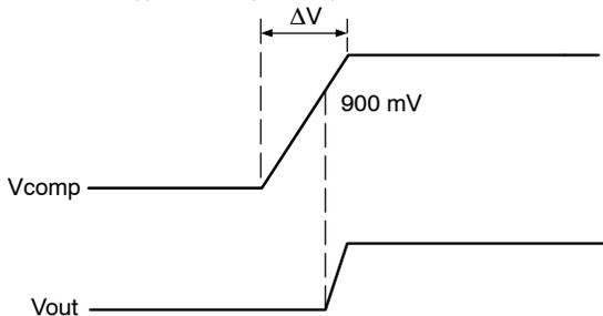
The above calculation includes the delay from comp rising to when output voltage starts becomes valid.
