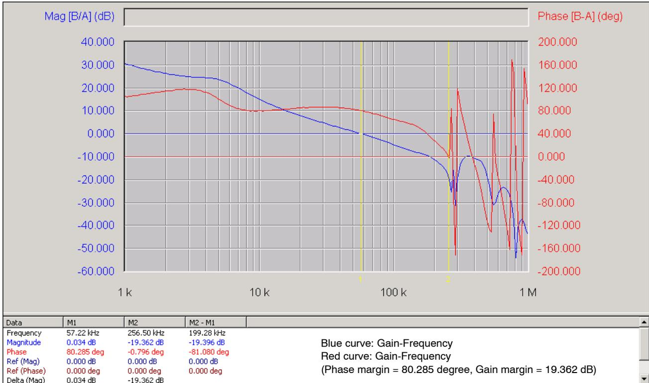
**Figure 14. Closed-loop Voltage Loop-gain of the NCP1587E**
