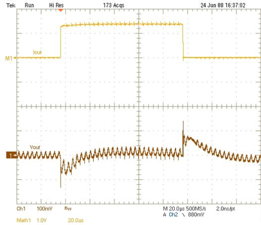
Figure 19. Transient Response 0-10 A Load Step
