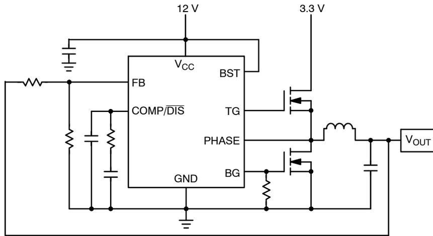
Figure 1. Typical Application Diagram
