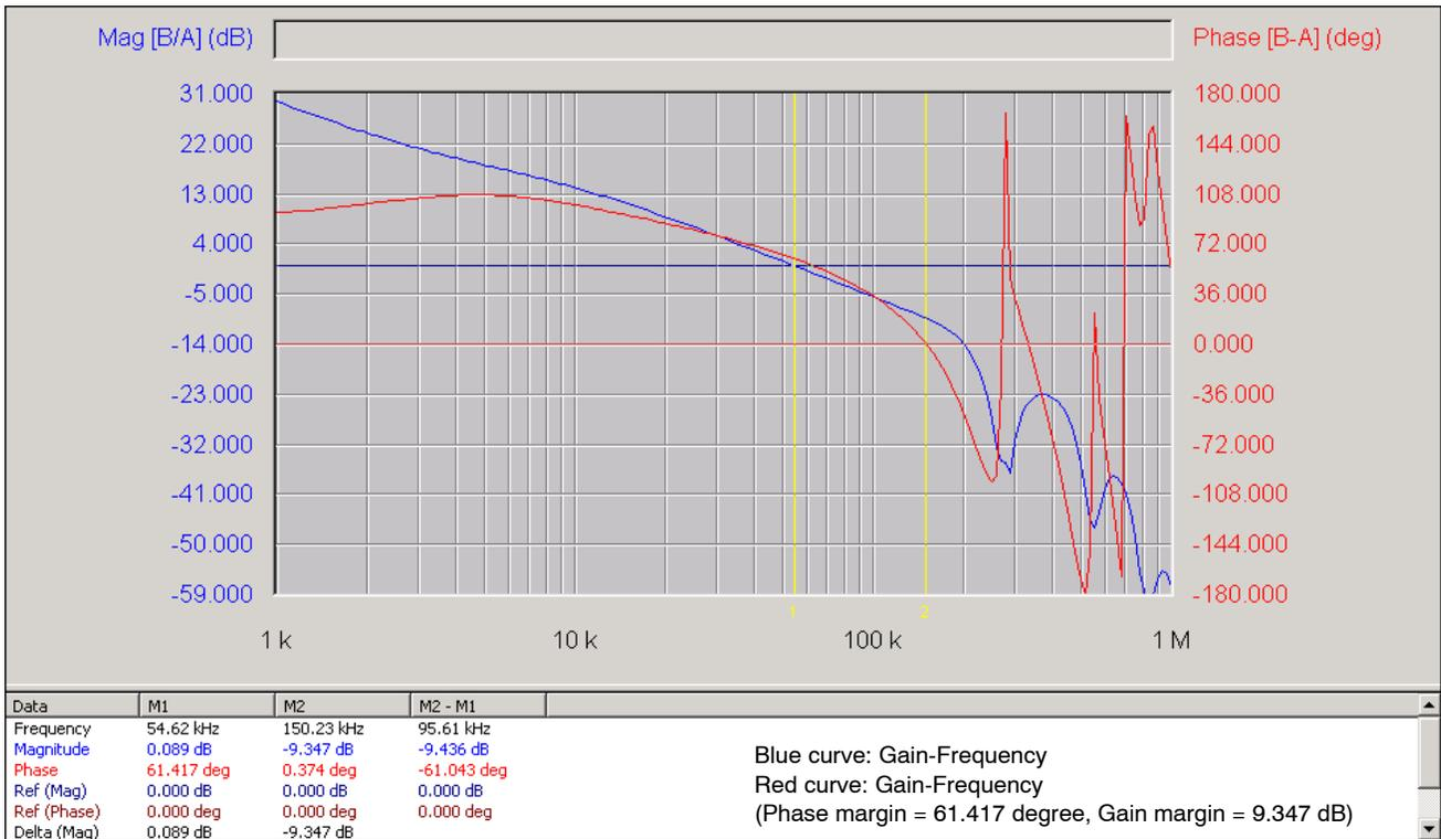
Figure 13. Closed-loop Voltage Loop-gain of the NCP1587E
