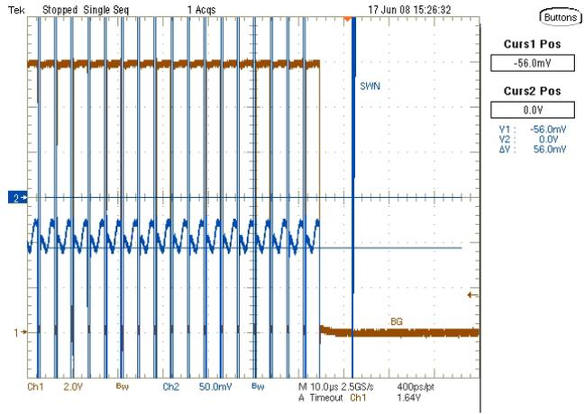
Figure 17. Over Current Protection (12.4 A DC Trip)
