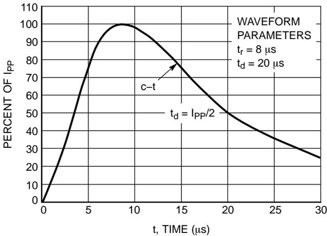
Figure 1. Pulse Waveform
