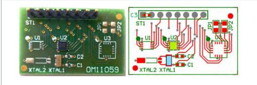
Fig 3. Picture and layout of demo bard OM11059
