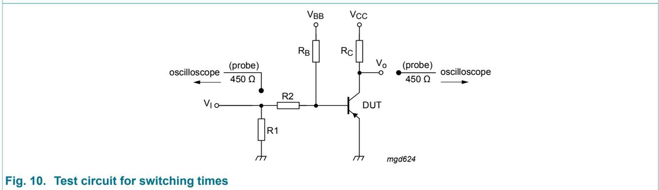
Fig. 10. Test circuit for switching times
