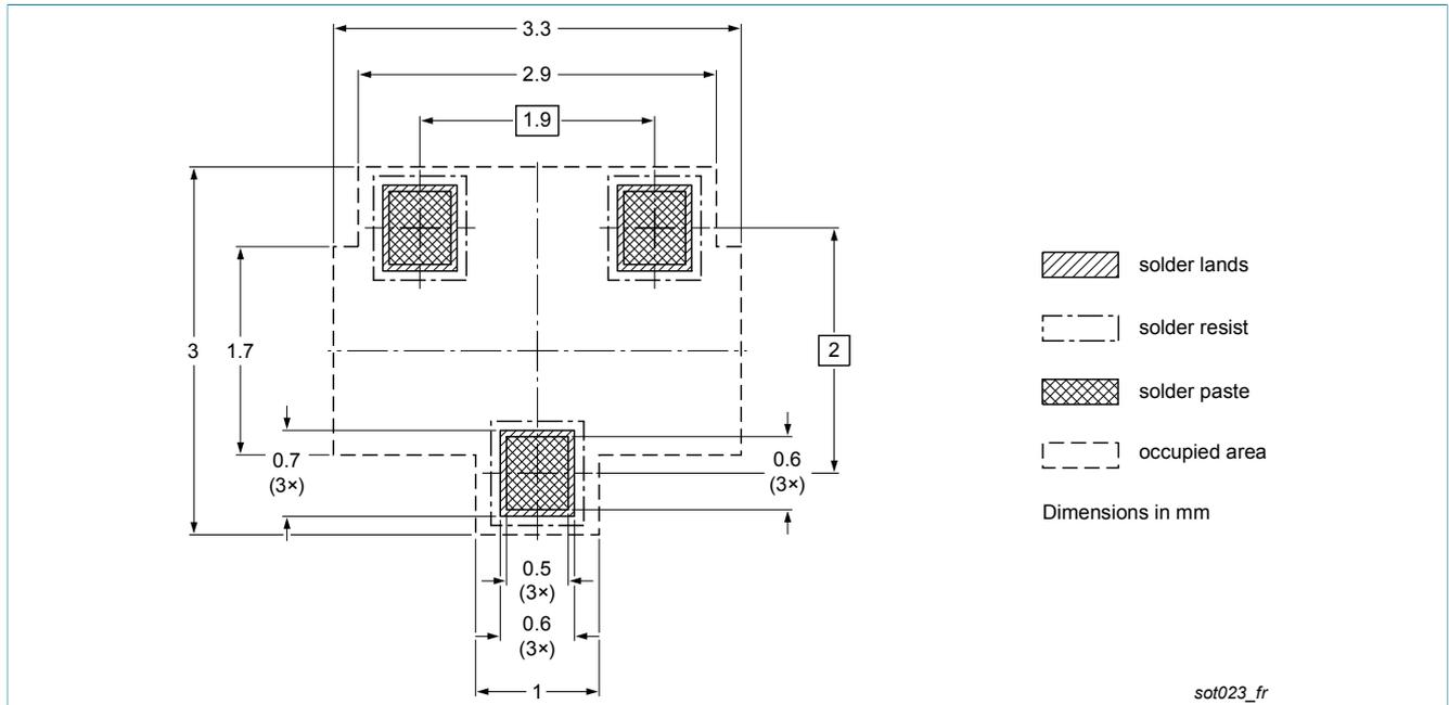
Fig. 12. Reflow soldering footprint for TO-236AB (SOT23)
