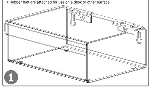
Mount securely to a wall with screws approved and supplied by building maintenance.
