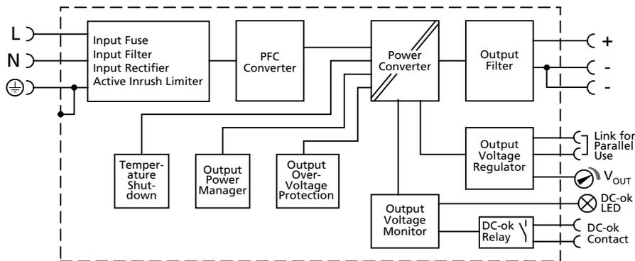
Fig. 11-3 **Functional diagram CP20.241-V1**
