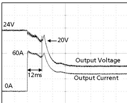
Please note: The DC-OK relay might trigger when the voltage dips more than 10% for longer than 1ms.
