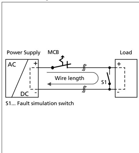
Maximal wire length<sup>\*)</sup> for a fast (magnetic) tripping:
