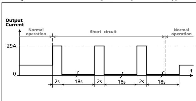
Fig. 6-4 **Dynamic overcurrent capability, typ.**
