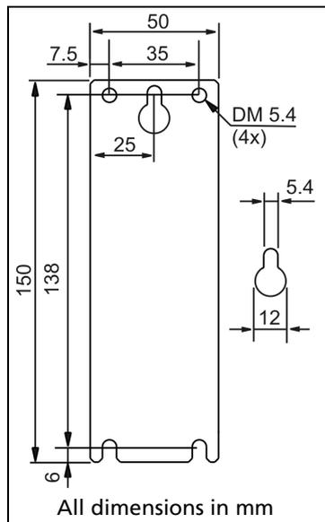
Fig. 23-6 **Wall/panel mounting, side view**
