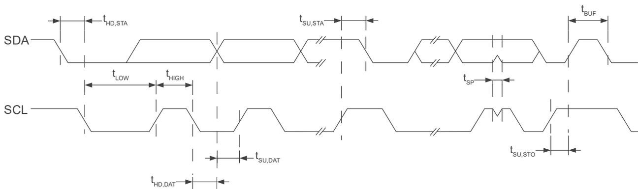
Figure 4.2: I<sup>2</sup>C Mode Timing Diagram
