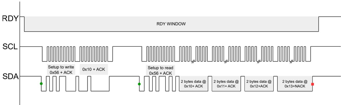
Figure 9.1: Example of Reading Data over I<sup>2</sup>C
