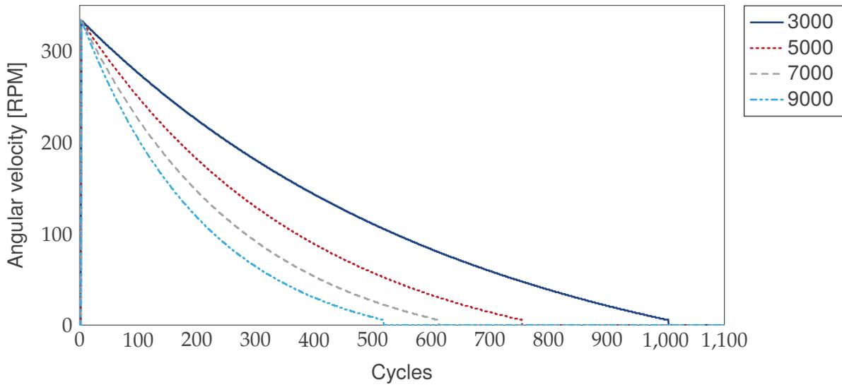
Figure 8.2: Freewheel Response as Damping Changes
