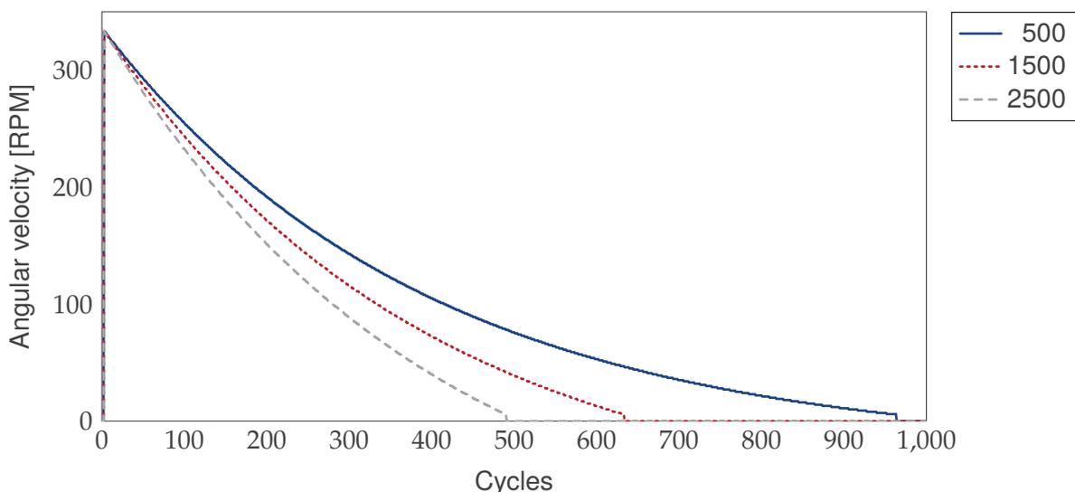
Figure 8.1: Freewheel Response as Friction Changes
