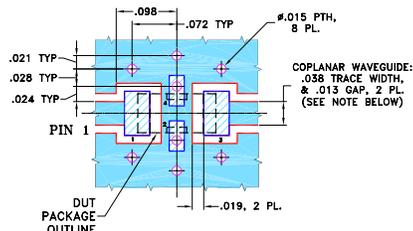
NOTES: 1. COPLANAR WAVEGUIDE PARAMETERS ARE SHOWN FOR ROGERS RO4350B WITH THICKNESS .020" ± .0015". COPPER: 1/2 OZ. EACH SIDE. FOR OTHER MATERIALS TRACE WIDTH & GAP MAY NEED TO BE MODIFIED.
