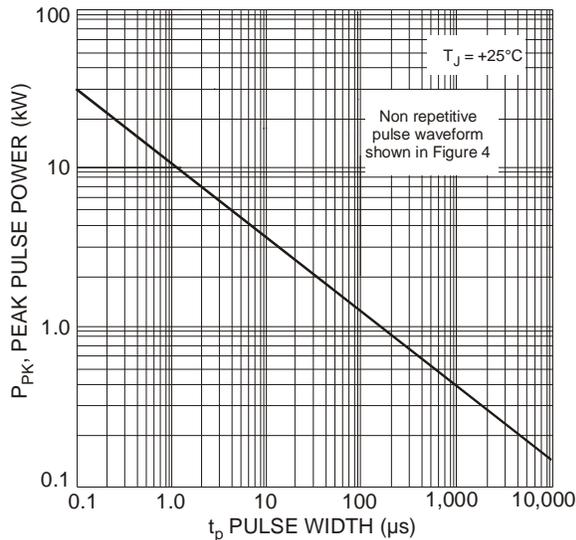
Figure 3 Pulse Rating Curve
