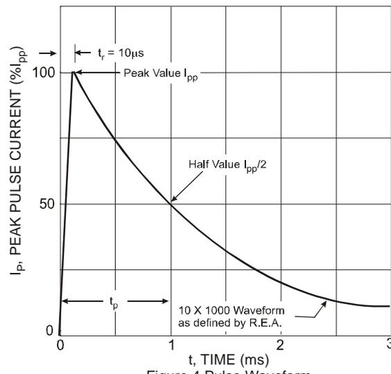
Figure 4 Pulse Waveform
