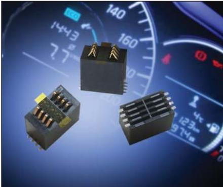
AVX extends their range of board-to-board stacker connectors used to connect two PCB's, with a new tall version 00-9148. This new connector is designed to connect 2 parallel boards using a 1-piece connector design for board spacing of 8mm in a double row configuration offering 8 positions at 1mm pitch. With a rated current of 1A continuous through each contact.
