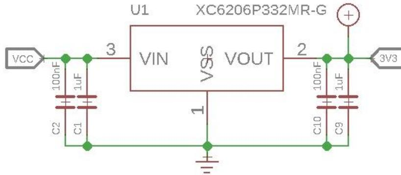
The typical voltage of AMG8833 is 3.3V, so we use the [XC6206P33](#) chip to provide a stable 3.3V. The input of XC6206P33 ranges from 1.8V to 6.0V, so you can use this module with your Arduino both in 3.3V and 5V.
