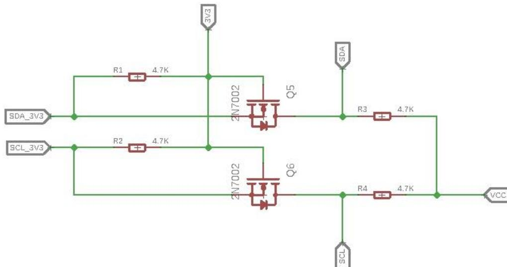
This is a typical Bi-directional level shifter circuit to connect two different voltage section of an I<sup>2</sup>C bus. The I<sup>2</sup>C bus of this sensor use 3.3V, if the I<sup>2</sup>C bus of the Arduino use 5V, this circuit will be needed. In the schematic above, **Q6** and **Q5** are N-Channel MOSFET [2N7002A](#), which act as a bidirectional switch. In order to better understand this part, you can refer to the [AN10441](#)
