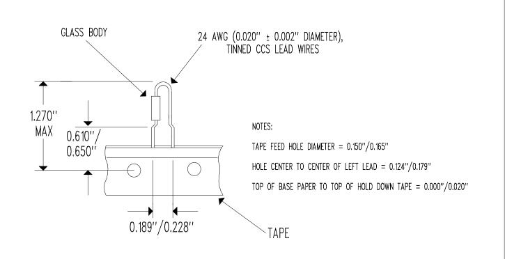
RESISTANCE @  $+25^{\circ}\text{C} = 10,000 \ \Omega \pm 10^{\circ}$ RESISTANCE TEMPERATURE CURVE = "J"
