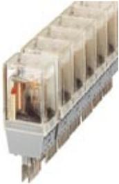
Relay connector, equipped with Siemens KAMMRELAIS ®, contacts (Ag): medium loads, 2 PDT, input voltage 24 V DC, with light indicator, can be plugged on basic termination blocks
