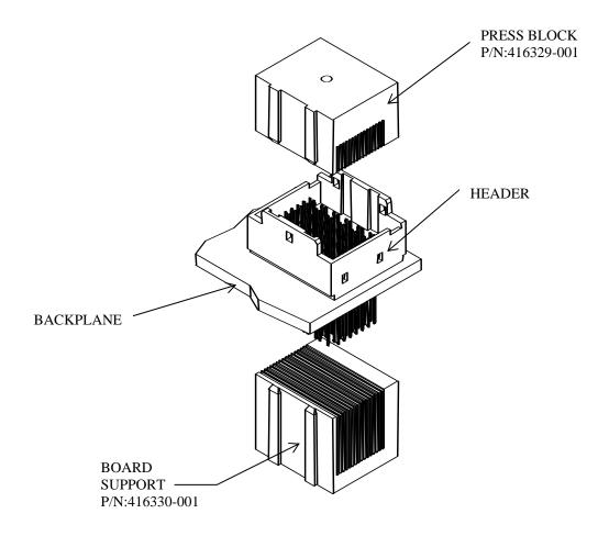
IF YOUR BACKPLANE IS GREATER THAN 4.30mm AND YOU ARE USING DASH NUMBERS X01, X02, AND X03 YOU WILL NOT NEED BOTTOM TOOLING AS THE TAIL WILL NOT EXTEND BELOW THE PC BOARD. IF YOUR BACKPLANE IS LESS THAN 4.30mm OR YOUR TAIL LENGTH IS GREATER THAN YOUR BACKPLANE YOU WILL NEED TO USE BOTTOM TOOLING.
