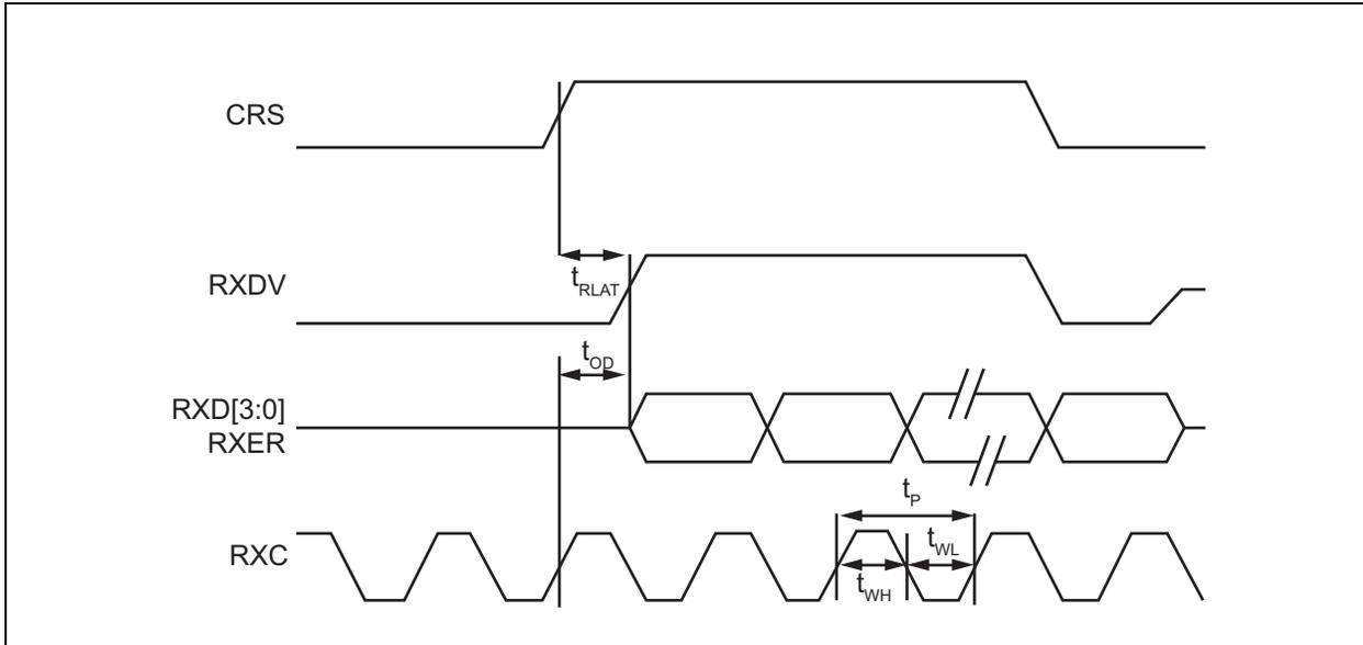
TABLE 7-3: MII RECEIVE TIMING (10BASE-T) PARAMETERS
