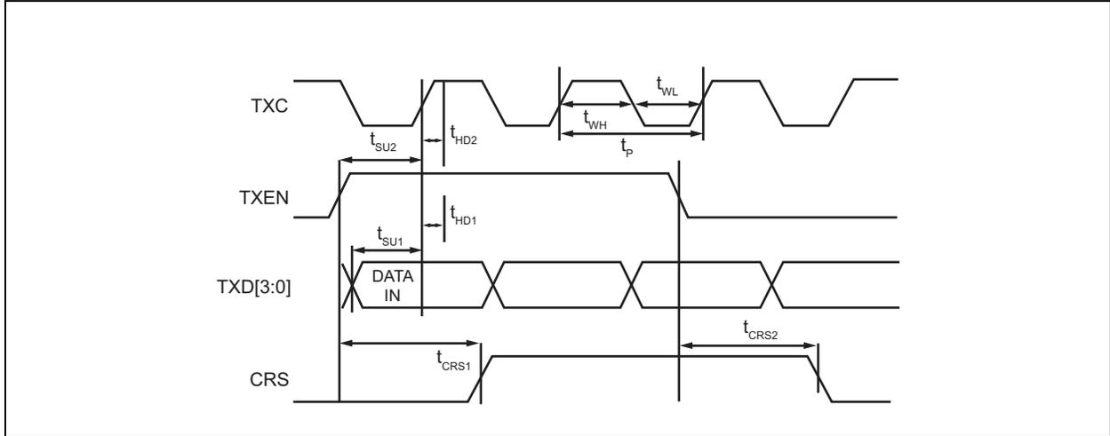
TABLE 7-4: MII TRANSMIT TIMING (100BASE-TX) PARAMETERS
