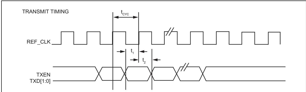
**FIGURE 7-7: RMII TIMING - DATA INPUT TO RMII**
