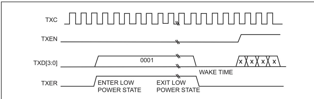
Similarly, the KSZ8091RNB enters LPI mode for the transmit direction when its attached IEEE-compliant RMII MAC de-asserts TXEN and sets TXD [1:0] to 01. The KSZ8091RNB remains in the LPI transmit state while the RMII MAC maintains the states of these signals. When the RMII MAC changes any of the TXEN or TX data signals from their LPI state values, the KSZ8091RNB exits the LPI transmit state.
