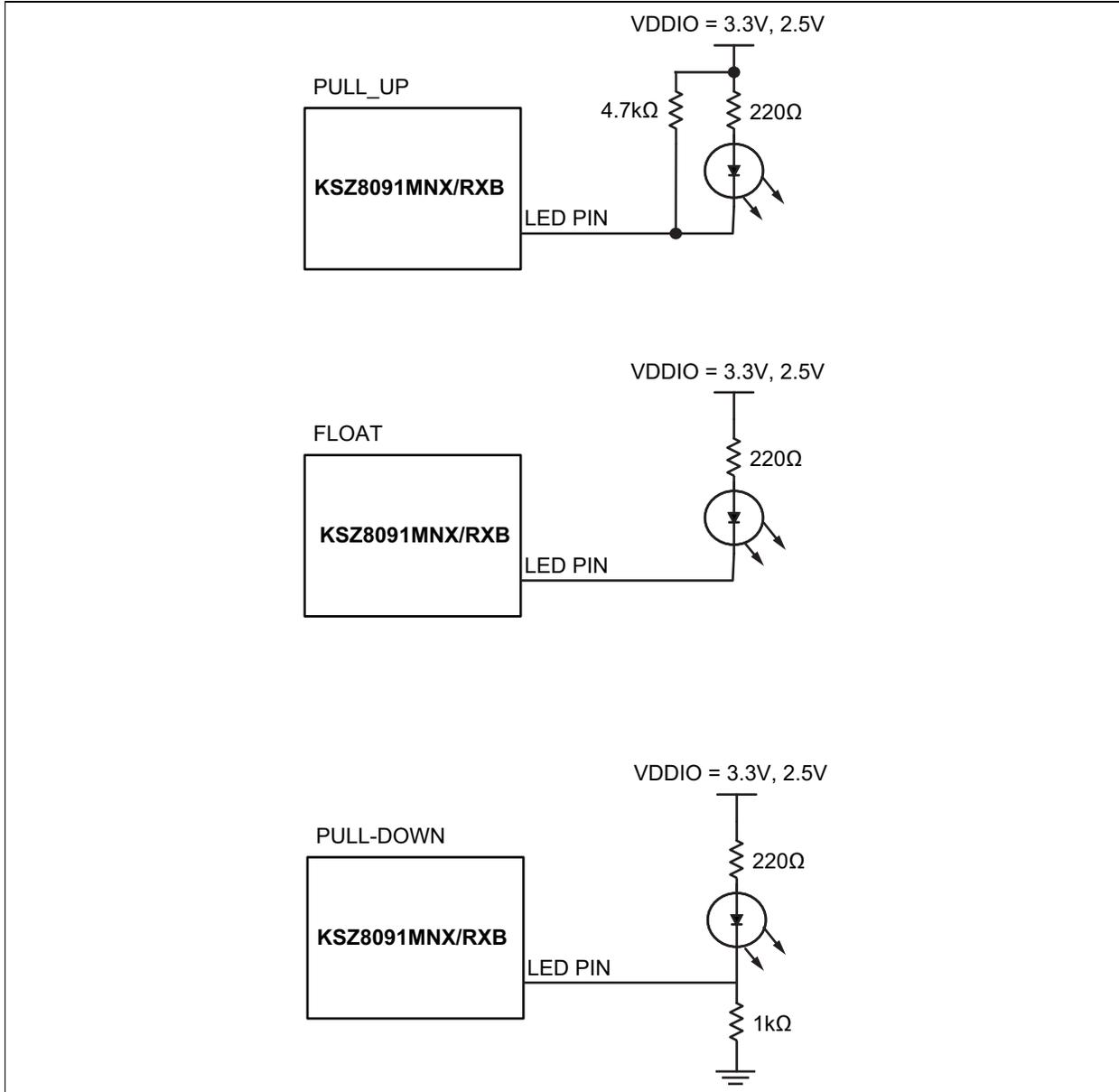
For 1.8V  $V_{DDIO}$ , LED indication support is not recommended due to the low voltage. Without the LED indicator, the SPEED and NWAYEN strap-in pins are functional with a 4.7 kΩ pull-up to 1.8V  $V_{DDIO}$  or float for a value of '1', and with a 1.0 kΩ pull-down to ground for a value of '0'.
