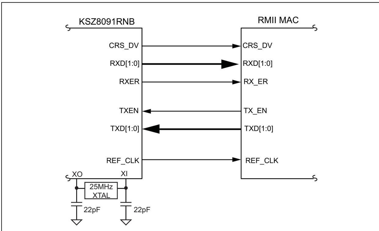
**FIGURE 3-4: KSZ8091RNB RMII INTERFACE (50 MHz CLOCK MODE)**
